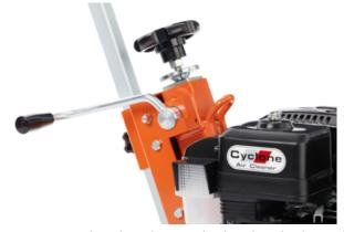
Automatic reset to the selected cutting depth and quick release of the drum from the ground.
