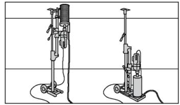
Drilling upwards and downwards.
