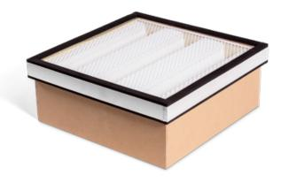
A large filter area in combination with pre-separation give long operation time with high efficiency. A pre-filter made of pleated polyester catches the larger dust fractions before the air enters the individually tested HEPA H13 filter ensuring 99.99% efficiency at 0.3 microns.
