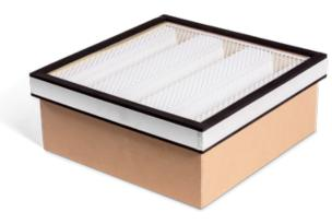
A large filter area in combination with pre-separation give long operation time with high efficiency. A pre-filter made of pleated polyester catches the larger dust fractions before the air enters the individually tested HEPA H13 filter ensuring 99.99% efficiency at 0.3 microns.
