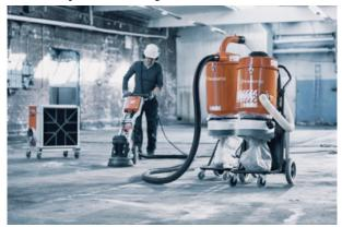
The pre-separator prolongs the dust extractors filter life and maintains higher airflow over time resulting in greater dust pick up, a cleaner work environment and longer time between filter cleaning.
