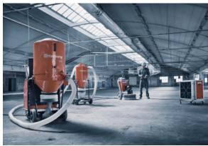
The pre-separator prolongs the dust extractors filter life and maintains higher airflow over time resulting in greater dust pick up, a cleaner work environment and longer time between filter cleaning.
