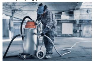
The powerful evacuation pump is capable of pumping the slurry 9 metres vertically or 200 metres horizontally.
