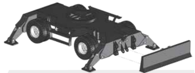
Heavy Duty 3000 mm-wide undercarriage with rear and front outriggers (optional blade)
