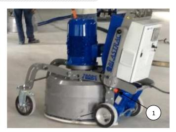
Clean the brush-sealing directly after wet grinding. It will be very hard to clean the brush-sealing when the dust-water mixture has dried up and hardened.
