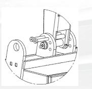
Use two pins when you tilt the machine back
