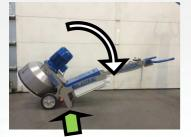
Remove the key of the dead man's switch, press the red stop button, and unplug the machine from the power supply.
