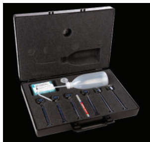
PENETRATION TEST KARSTEN PIPE TEST KIT 598 85 80-02
