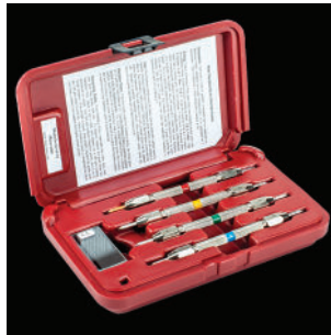
HARDNESS TEST MOH'S TEST KIT 593 31 69-01
