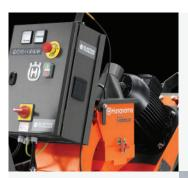
**Option of 1 or 3 phase** This heavy duty professional machine is available either in 230 V (easy to plug on most jobsites) or 400 V.
